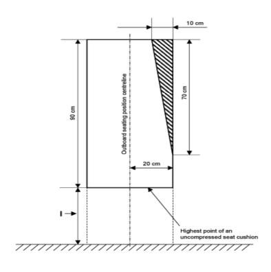
1 (cm) min. 40-50 (35 cm at wheel arches and engine compartment)
