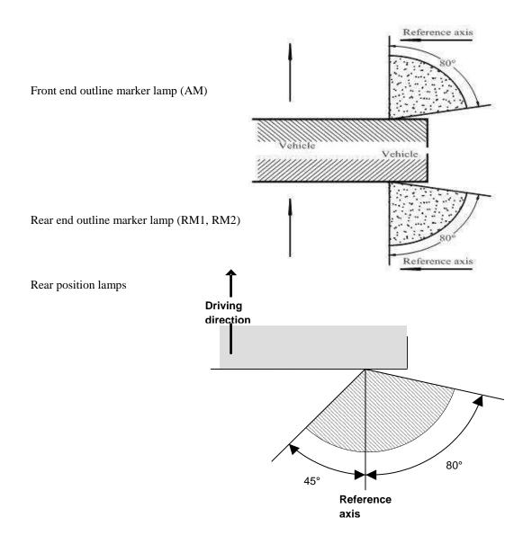
Under the H plane for rear position lamps intended to be installed with this plane at a mounting height less than 750 mm above ground.
