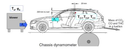
■ Interior: measured TV3-3,4 for vent and TC1,3 for cabin
