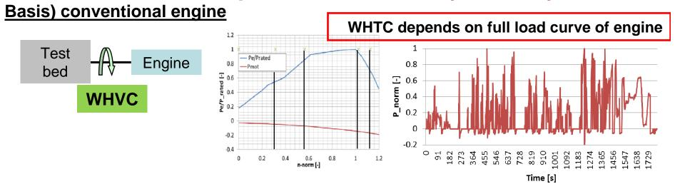
WHDC = reference for typical load distributions for HDV driving
