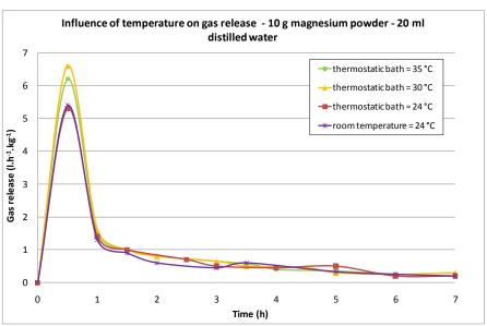
if there is a possibility of self-heating when material is transported in bulk, it seems relevant to perform another test at a higher temperature
