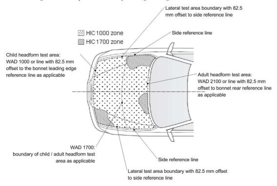
Figure 11: Example of marking of HIC1000 zone and HIC1700 zone
