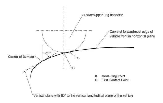
Figure 6C: Measuring and first contact point (see paragraphs 3.31. and 3.19.)
