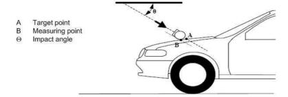
Figure 6A: Measuring Impact and target point in the vertical longitudinal plane through the center of the impactor (see paragraphs 3.30. 3.19. and 3.25.) \*)
