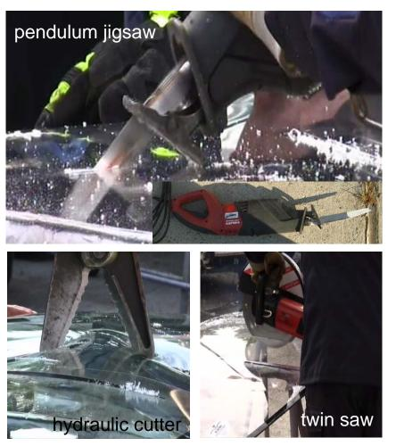
... pendulum jigsaw, twin saw, cut-off grinder and hydraulic cutter can be used without any difficulty to cut polycarbonate glazing. ...
