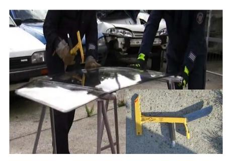
...different compared to glass. ... spring center punch, glass saw or Hooligan tool (special forcible entry tool) are not useful...
