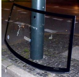
...during the rescue work it was possible to remove the intact PC windscreen from KRD in one piece.
