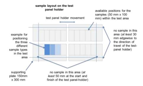
This assures that the test samples are located in the optimal testing area of the test apparatus. The area of at least 50 mm at the start and finish of the test-panel holder and of at least 30 mm edgewise to the direction of travel of the test-panel holder may not be evaluated.
