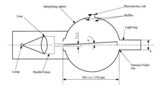
For the *measurement* place the test piece against the entrance port of the integrating sphere. The angle between the normal (perpendicular) to the surface of the test piece and the axis of the light beam shall not exceed 8°.
