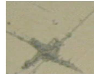
Figure 5. CCD image of the ExatecPlus surface after the Taber test showing severe damage at intersections of scratches.
