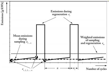
The system test of a periodically regenerating particulate reduction REC is considered passed if the [nominal] particulate emissions calculated using the procedure set out below are within the limit set for the reduction level for which the applicant wishes the REC to be approved.
