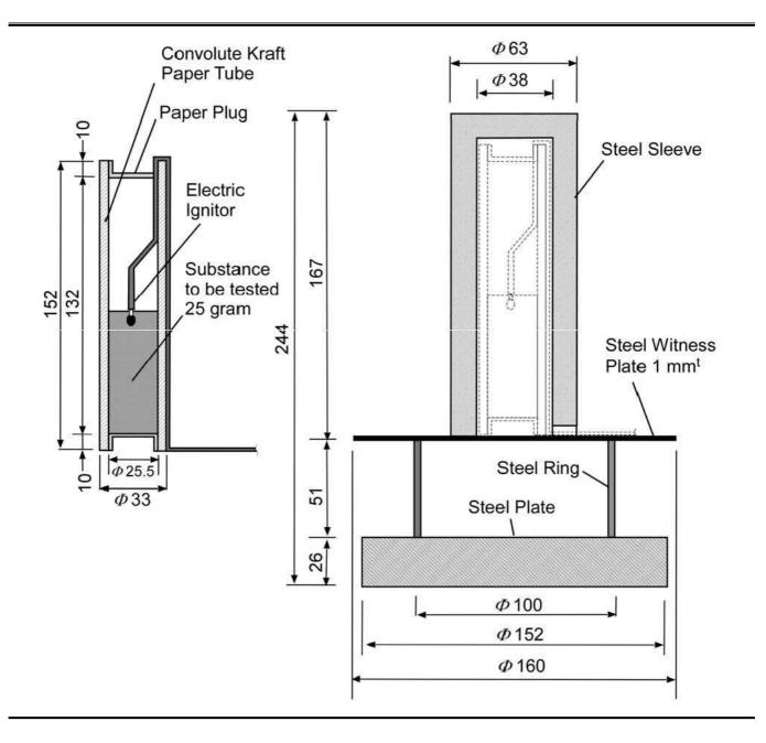
Figure 1: <u>DDT</u> Flash Composition Test Apparatus Drawing
