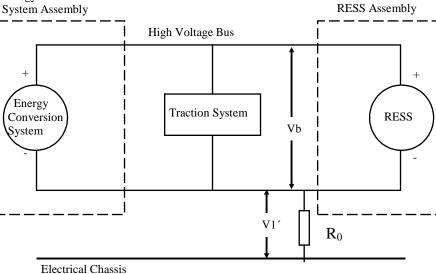
Figure 2: Measurement of V1'
