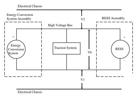
Figure 1: Measurement of Vb, V1, V2
