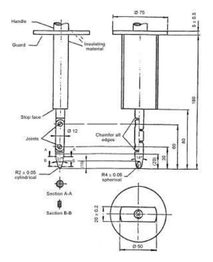
Material: metal, except where otherwise specified Linear dimensions in millimeters Tolerances on dimensions without specific tolerance:
