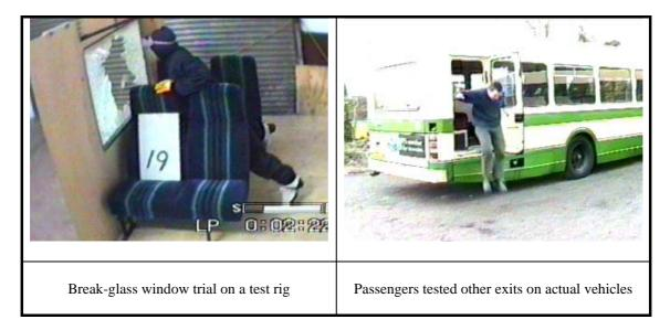
The results show that the design of the opening mechanism has a far greater effect on exit times than, for example, whether the door is a service, emergency or 'continental' door. With good operating mechanisms doors can be the quickest exits to use. While hinged windows are only marginally slower than doors, break-glass windows can take up to 6 times longer due to the time taken to clear the glass from the frame.
