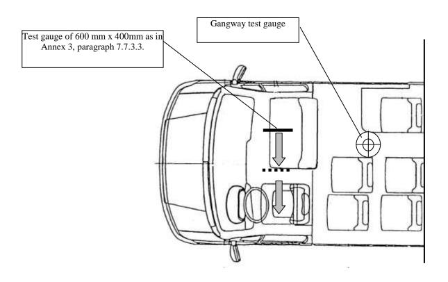
Up to five additional seats may be fitted in a compartment incorporating the driver's compartment, provided that the additional seats and the space for these seats comply with all requirements of this Regulation and at least one door giving access to the passenger compartment complies with the requirements of paragraph 7.6.3. for emergency doors.
