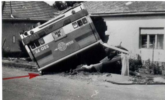
Figure 1. General collapse of the superstructure in rollover
