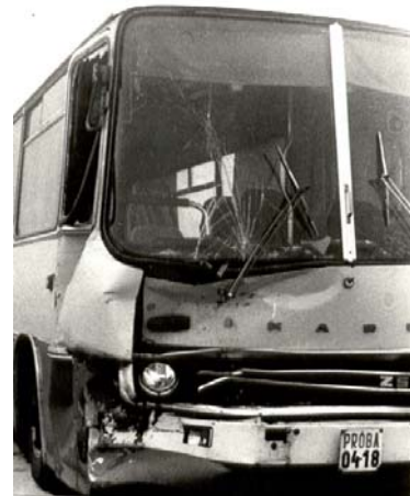
Figure 2. Local large-scale deformation of the bodywork
