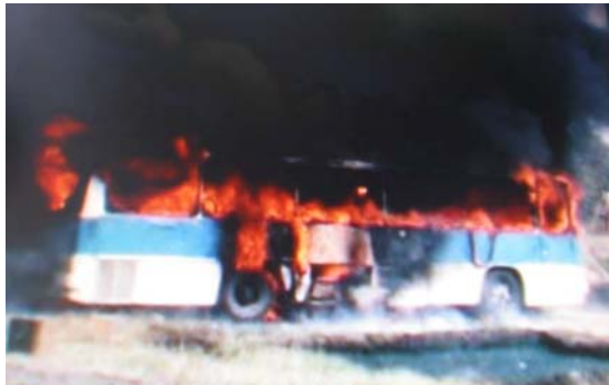
Figure 3. Fire tests with complete bus type IK255
