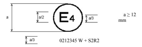
The above approval mark shows that the tyre concerned has been initially approved in the Netherlands (E4) pursuant to Regulation No. 117 and the 02 series of amendments under approval number 0212345. This indicates that the approval is for W (wet grip). The S2R2 preceded by + indicates that it has had its approval extended under Regulation No. 117 to rolling sound at stage 2 and rolling resistance at stage 2 based on separate certificate(s).
