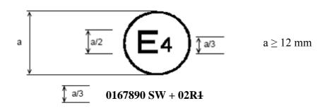
The above approval mark shows that the tyre concerned has been initially approved in the Netherlands (E4) pursuant to Regulation No. 117 and the 01 series of amendments under approval number 0167890. This indicates that the approval is for S (rolling sound at stage 1) and W (wet grip). The 02R4 preceded by + indicates that it has had its approval extended under Regulation No. 117 and the 02 series of amendments to rolling resistance at stage 1 based on separate certificate(s).
