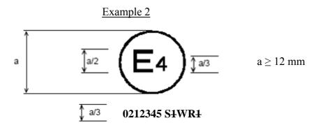
The above approval mark shows that the tyre concerned has been approved in the Netherlands (E4) pursuant to Regulation No. 117 (marked by **S1** (rolling sound at stage 1) W (wet adhesion), and R1 (Rolling resistance at stage 1) under approval number 0212345. This indicates that the approval is for S1WR1. The first two digits of the approval number (02) indicate that the approval was granted according to the requirements of the 02 series of amendments of this Regulation.
