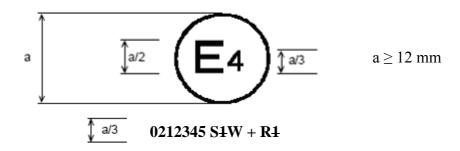
The above approval mark shows that the tyre concerned has been initially approved in the Netherlands (E4) pursuant to Regulation No. 117 and the 02 series of amendments under approval number 0212345. This indicates that the approval is for S4 (rolling sound at stage 1) and W (wet grip). The R4 preceded by + indicates that it has had its approval extended under Regulation No. 117 to rolling resistance at stage 1 based on separate certificate(s).
