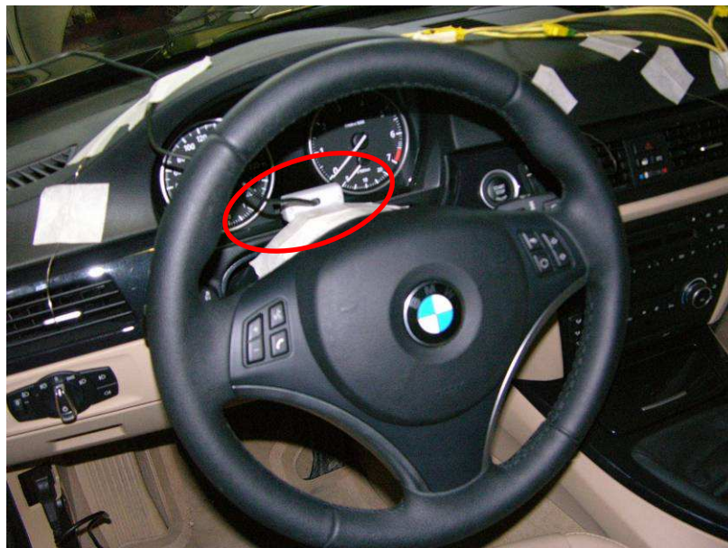
Figure 41: Camera to transfer the signal of the gear shift indicator to the driver's aid
