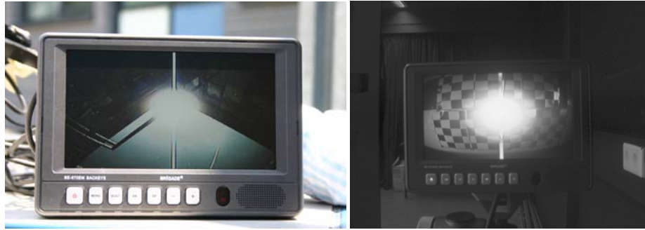
Figure 2. a) shows the blooming area outdoors in broad daylight (sun illumination of 93500lx) compared to blooming area under test conditions in the lab (b). The blooming area in the latter case is larger (10% compared to 6%) but comparable; the blooming area is defined by the region in which no black squares can be detected (luminance contrast lower than 0.20).
