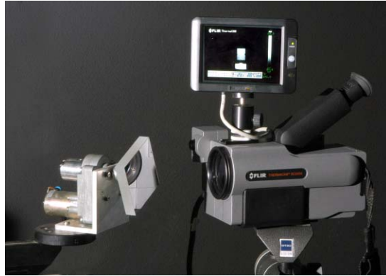
Figure 10. Setup with a rotating mirror in front of the camera which may be used for dynamic TOD testing.
