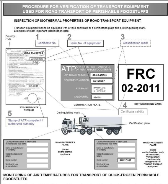
The transport equipment must be fitted with a suitable recording instrument to monitor, at frequent and regular intervals, the air temperatures to which quick-frozen foodstuffs intended for human consumption are subjected.
