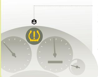
By 2008, all new vehicles will be equipped with a Tire Pressure Monitoring System to alert motorists to low tire pressure.
