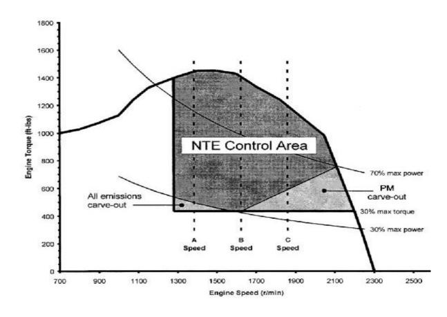
Figure 2. Example Not-To-Exceed Control Area When NTE C Speed > 2,400 rpm
