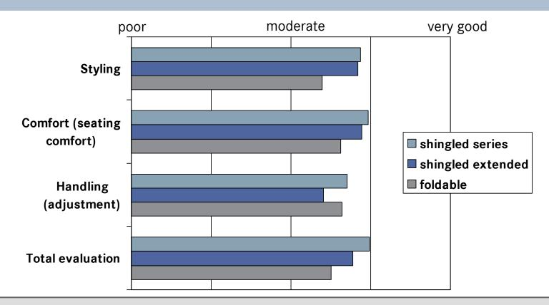
Altogether the series "shingled" head restraint is evaluated best (statistically significant better as the foldable head restraint). The "extended shingled" head restraint declines a little bit in handling. Raising up of the head restraint was too tight for many candidates (could have been a prototype problem?).
