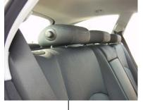
Success criteria: head restraint folded upwards
