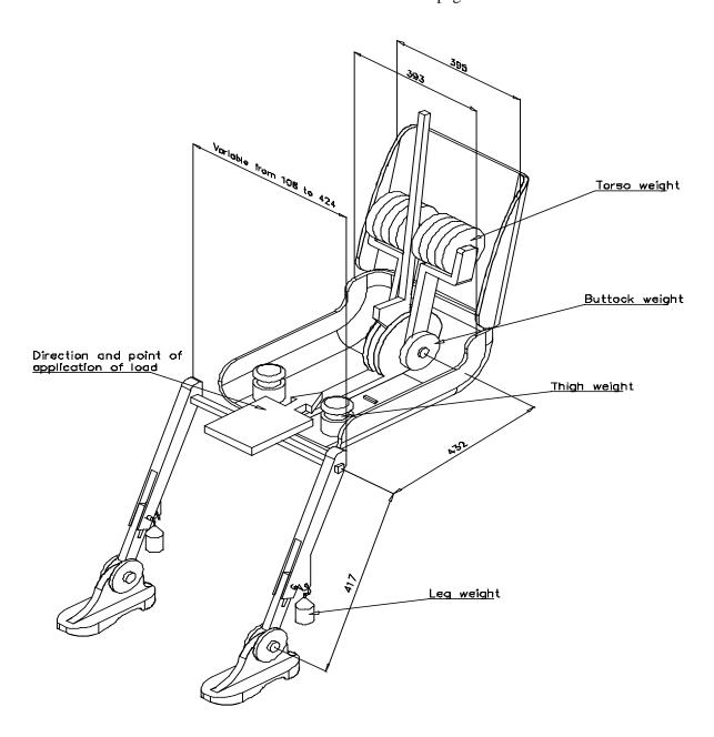
$\underline{\text{Figure 2}}$  - Dimensions of the 3-D H machine elements and load distribution (Dimensions in millimeters)
