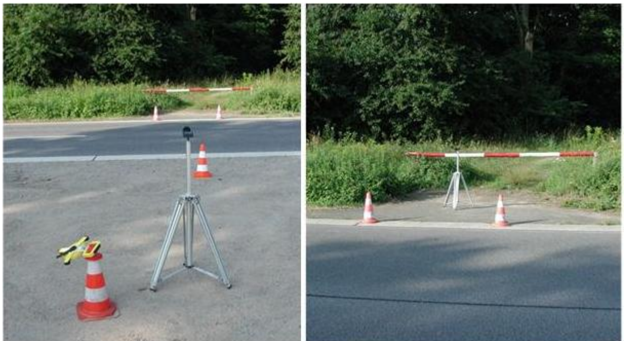
Figure 3: Microphone positions for a roadside enforcement test
