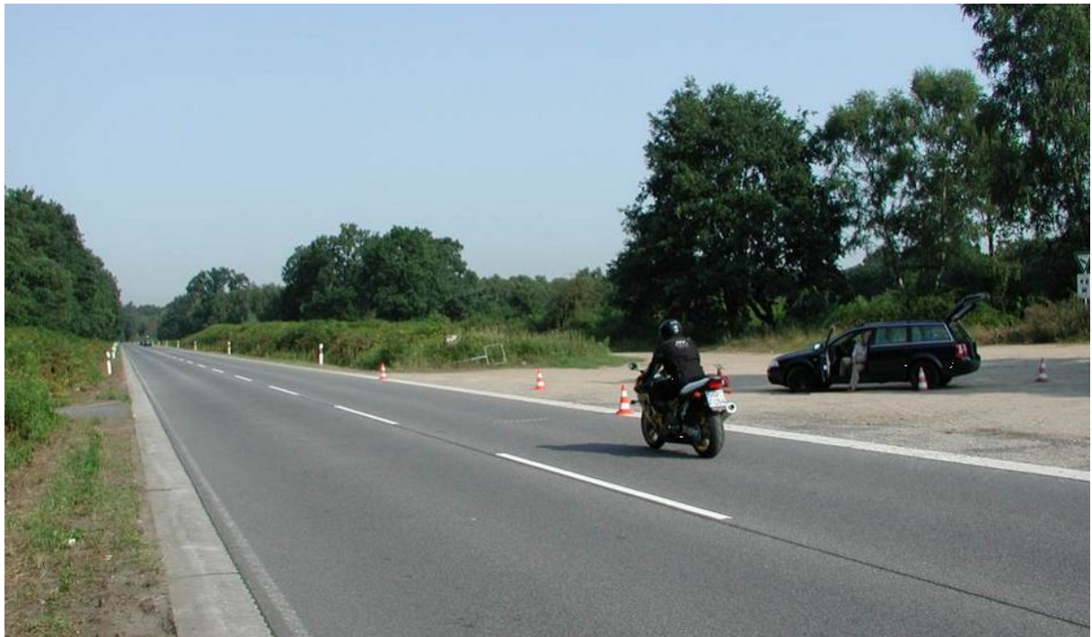
Figure 2: Example for a pass-by roadside enforcement test
