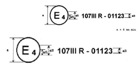
The above approval mark affixed to a vehicle shows that the vehicle type concerned has, with regard to its constructional features, been approved in the Netherlands (E 4) for Class III, pursuant to Regulation No. 107 under approval number 01123. The approval number indicates that the approval was granted according to the requirements of Regulation No. 107 as amended by the 01 series of amendments.
