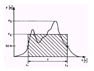
2.6. Clamping force  $F_c$  is the arithmetical mean value of the effective forces, measured at the same measuring point subsequently more times:
