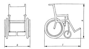
Overall length, l: 1200 mm Overall width, b: 700 mm Overall height, h: 1090 mm <u>Note</u>:
