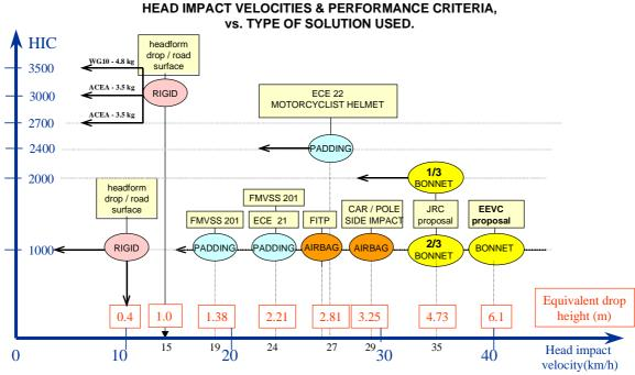
Consistently and confidently "passing" a legislative requirement like HIC less than 1000, at a head impact velocity of 40 km/h, with a "padding type" solution (car bonnet) seems to be out of reach. "State of the art" solutions to pass HIC less than 1000 at impact velocities of 25 to 29 km/h are airbags or other new developments.....
