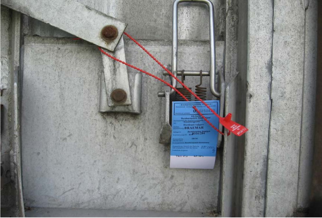
Photo 25: Use of a numbered tamper evident seal to close a bulk vehicle.
