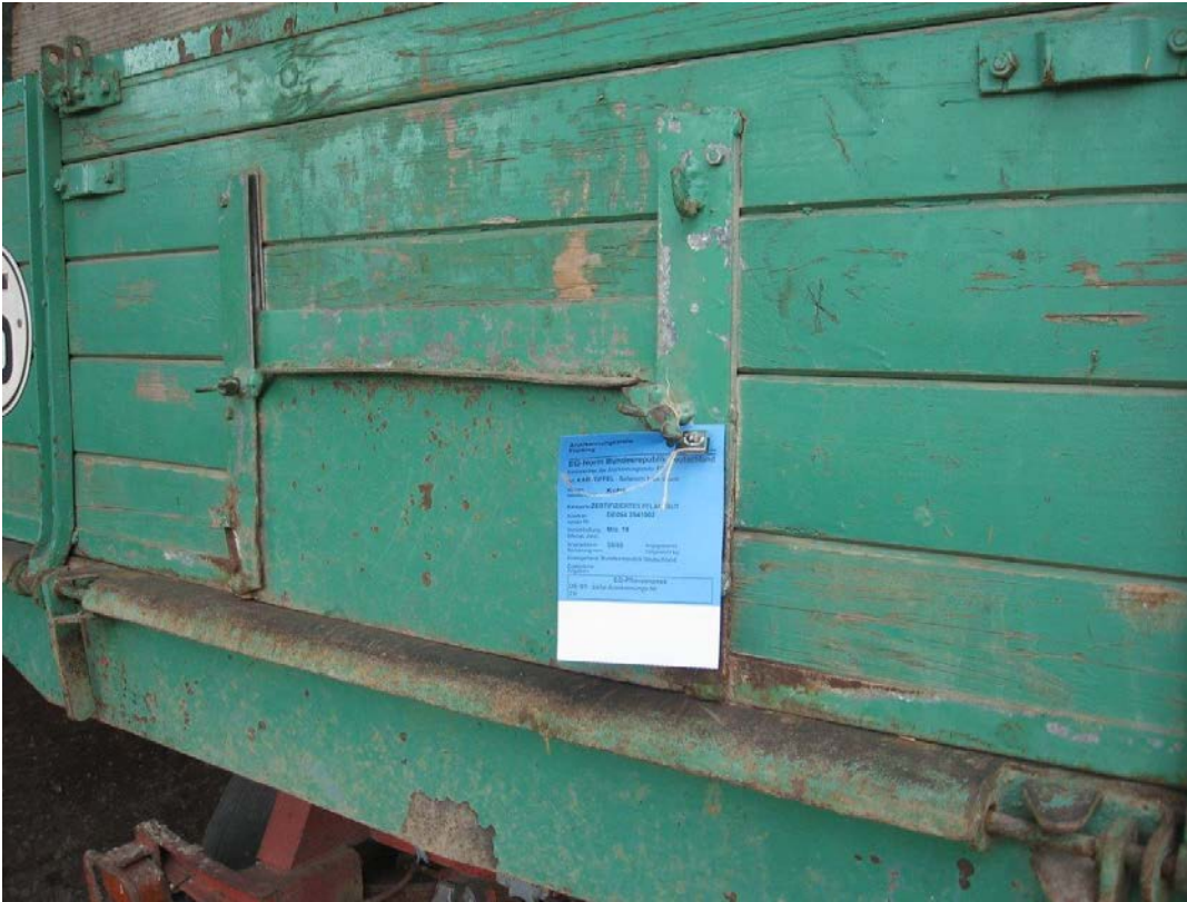
Photo 28: Use of tamper evident seal to close the tailgate of a vehicle carrying bulk bins.
