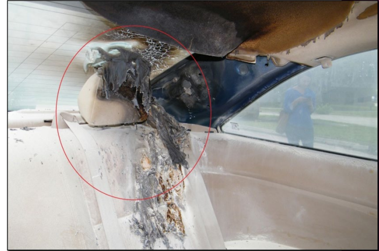
Interior View of Backseat/Headrest Area After Driver Side Airbag Inflator Ruptured
