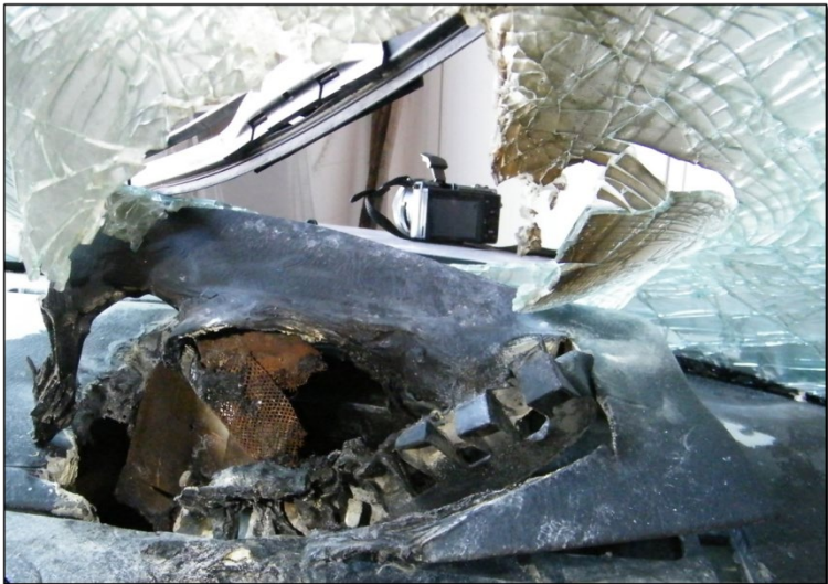
Passenger Side Airbag Inflator After it Ruptured
