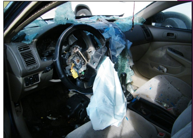
Driver Side Airbag Inflator After it Ruptured
