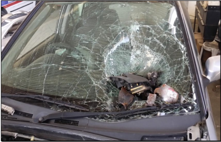
Exterior View of Windshield After Passenger Side Airbag Inflator Ruptured (RHD Vehicle)
