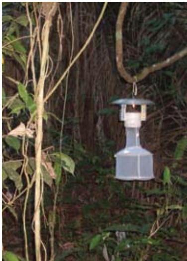
CDC trap capturing vectors of (re)emergent and neglected infectious diseases (Leishmaniasis and Bartonellosis). Photo by Manuel Cesario
