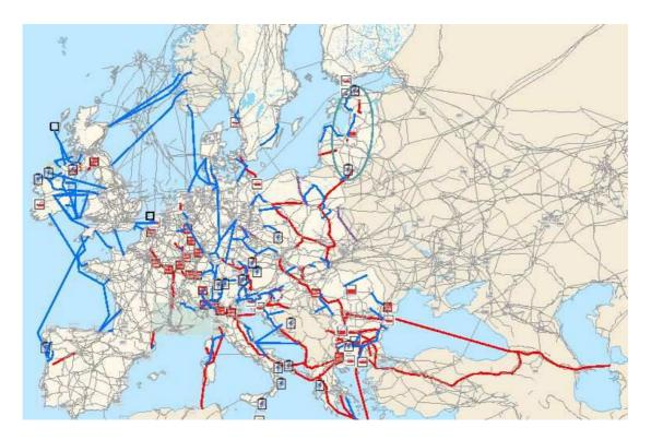
The scale of the Projects of Common Interest can be seen in the above Figure from the EU website – the blue being High Voltage Electrical Infrastructure and red being gas networks
