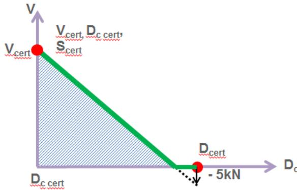
4.2. If the calculated performance value requirements fall within the hatched area of Figure 28, the towable mass is verified with a limiting V-value. For the combination concerned the limiting V-value overrules the certified V-value of the coupling equipment installed.
