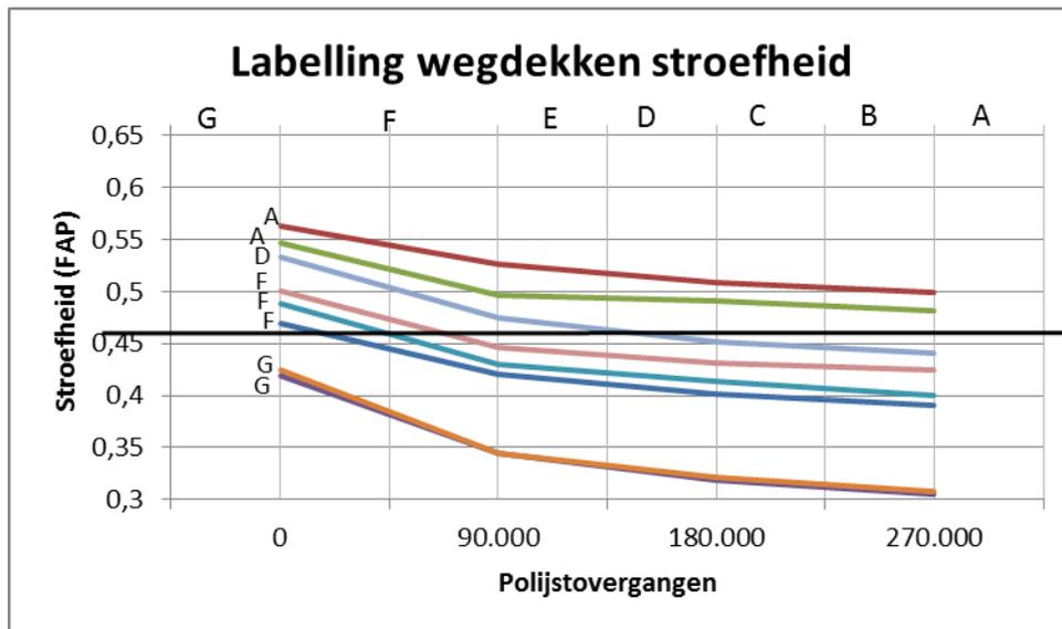
Further research into this experiment and the creation of a database with data from the FAP test for various mixtures and aggregate types is necessary to gain a good understanding of the differences in texture and composition of mixtures and the impact on dry skid resistance.
