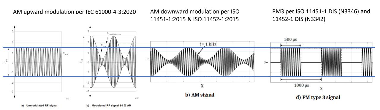
Peak conservation in ISO 11451-1 and 11452-1 ensures that the maximum amplitude level of AM does not exceed the maximum CW level while PM corresponds to a pulsed (i.e. on-off) CW signal.
