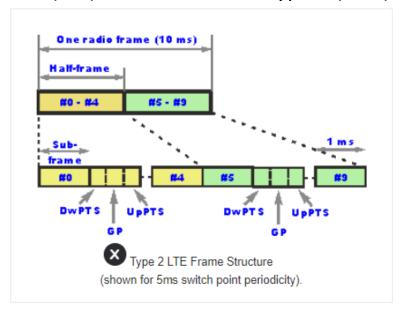
Frame length: 10ms (consisting of 10 sub-frames)
