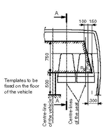
1 (b) LONGITUDINALLY Section A-A of the vehicle in the vertical plane of the centre-line of the inboard seat.
