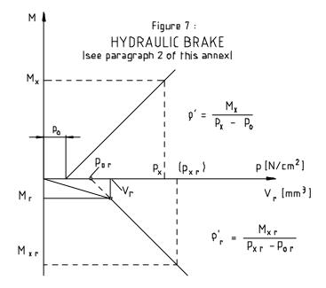
Figure 8: HYDRAULIC-TRANSMISSION BRAKING SYSTEM (see paragraph 2 of this annex)
