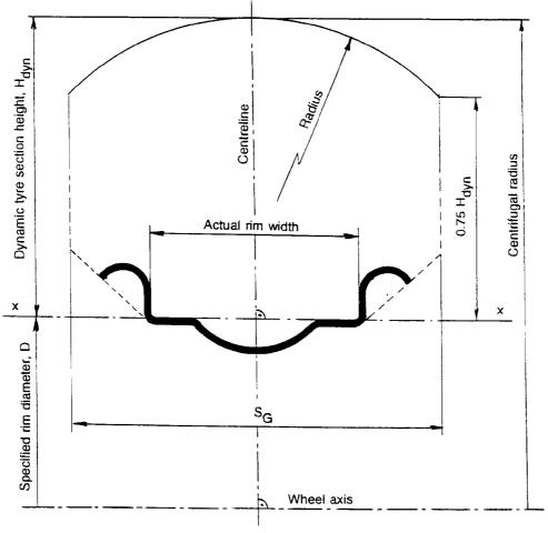
$S_{\mbox{\scriptsize G}}$  = Maximum overall width in service (This changes 1 mm per 0.1 Rim width code change from the measuring rim)
