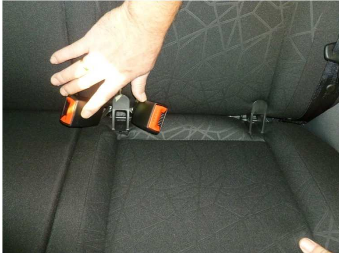
Buckle placed inside the ISOFIX anchorage distance
