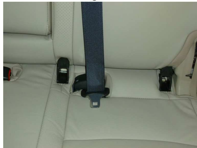
Buckle placed inside the ISOFIX anchorage distance
