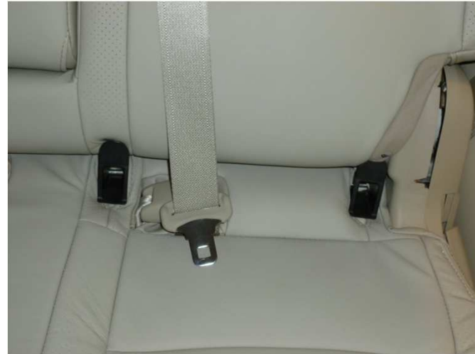
Buckle placed inside the ISOFIX anchorage distance
