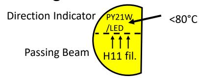
For H11/LED Substitutes, no "bottom heating", additionally the significant self-heating of the Halogen bulb removed
