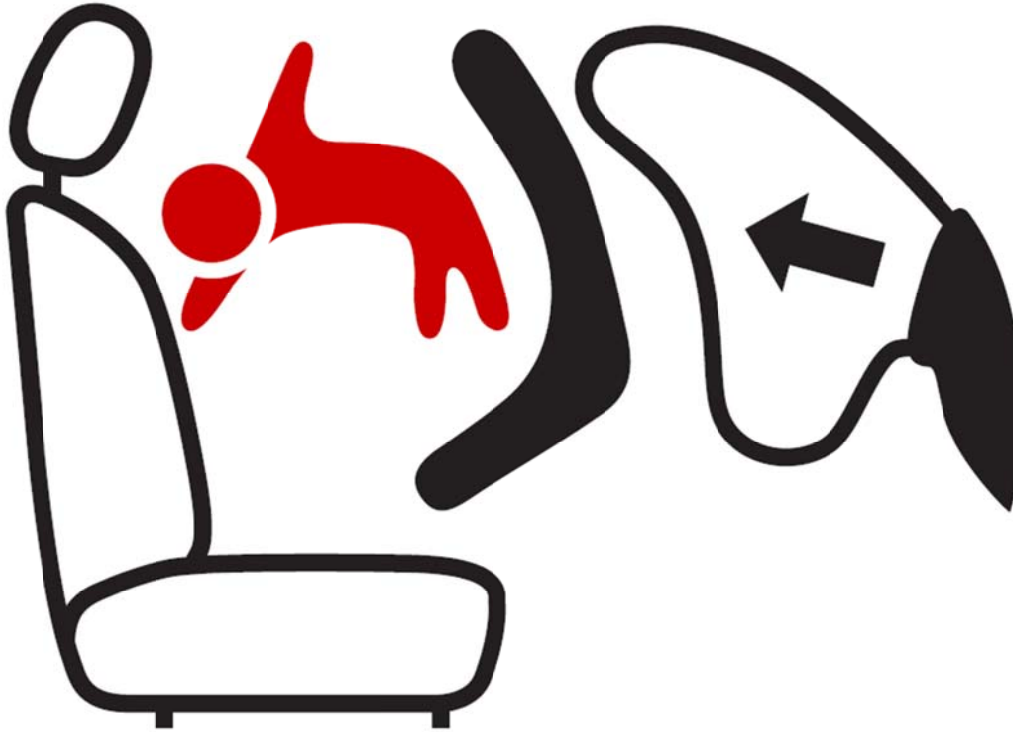
Figure C Pictogram depicting airbag deployment danger that shall be used and that shall measure 40 mm in width and 28 mm in height or proportionally larger
