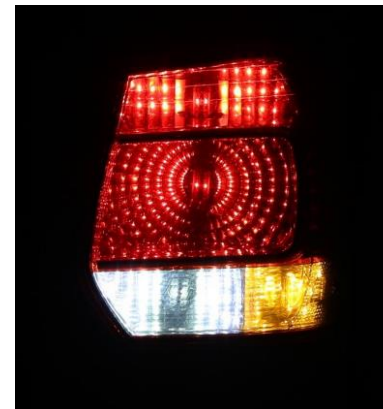
Philips LED Replacement Light Sources in VW Golf VI Variant rear light with clear cover
