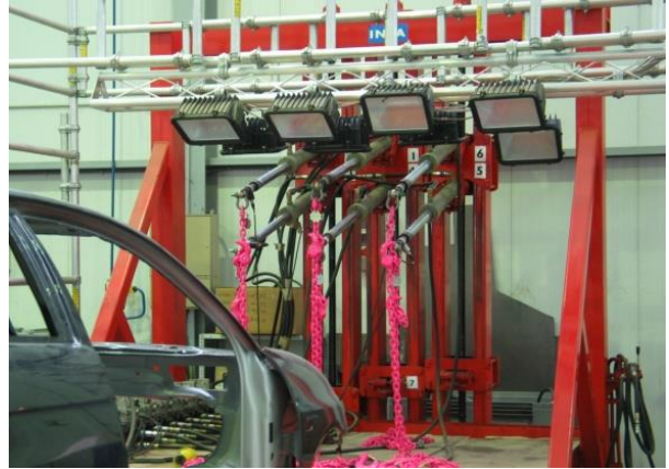
Testing machine for safety belt anchorages ©INTA - Spain Testing machine for seat anchorages ©INTA - Spain
