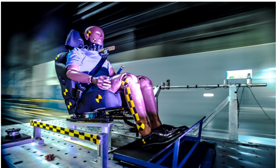
Inverse Catapult for testing safety belts© UTAC CERAM - France
