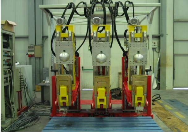
Testing machine for safety belt anchorages ©INTA - Spain Testing machine for seat anchorages ©INTA - Spain
