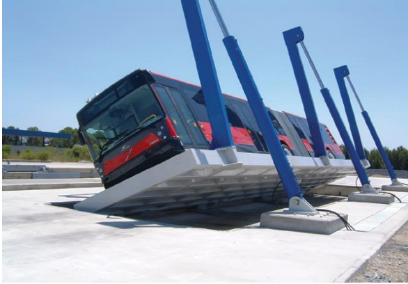
Testing coach superstructure resistance © IDIADA - Spain
