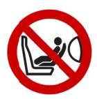
Figure 3 Pictogram depicting airbag deployment danger that shall be used and that shall measure 40 mm in width and 28 mm in height or proportionally larger
