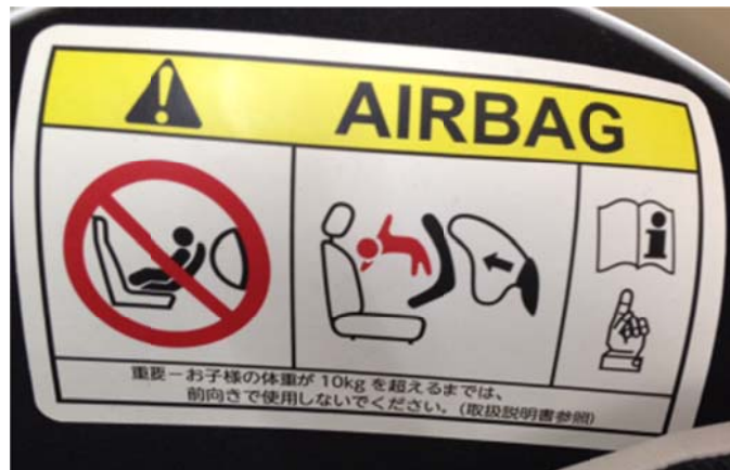
Label as found in the field with exact pictogram images and additional information outside the prescribed area
