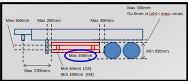
Loading requirement under <u>1kN force</u> application: displacement under <u>30mm or</u> 150mm depending on the force application location
