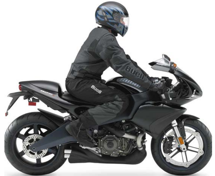
Motorcycle with Cockpit and Windscreen – Instruments Directly Face the Rider (sensor therefore in shadow)
