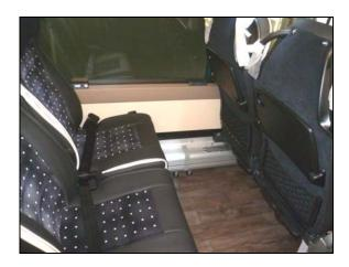
6. Generally the bottom of the squab of passenger seats is curved (especially for Class B and III vehicles) to provide best comfort to the occupants. The rear part of the new proposed gauge aims at reflecting the shape of the human back, and the radius of the front aims at simulating the rotation of the knees around the hips.
