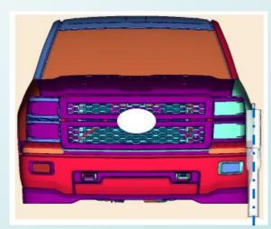
For this vehicle, an offset of 42 mm along the contour (as discussed in TF-BTA) would change the measuring point by 4 mm in y-direction
