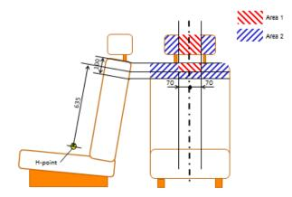
Reg.17, par. 6.8.1.1.3.(Area 1) + par. 6.8.1.2.2.(Area 2): In the case of seats with integrated head restraints
