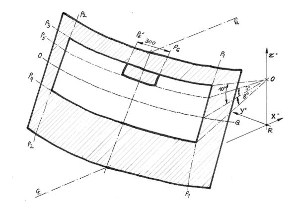
Measured on the outer surface of the windscreen and on the trace of plane 5. If this is not possible (in the absence of a symmetrical median longitudinal plane, for instance) P6 and P6′ shall be the planes parallel to the longitudinal plane of the vehicle passing through point 0."
