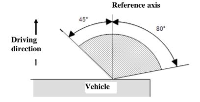
Under the H plane for lamps intended to be installed with this plane at a mounting height less than 750 mm above ground
